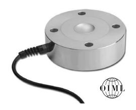
even when side forces are inevitable in normal operations. The typical example for side force resistance is the application in motor truck scales. PSD is constructed of alloy steel and is fully potted with special chemical compounds to IP67 to protect the cell from water and moisture attack.
